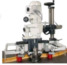
The Arc Feed Attachment type BV with its new feeding system allows the manufacturing of profiled, rebated, or curved strips or wooden work pieces on a standard spindle moulding machine with a vertical spindle.
