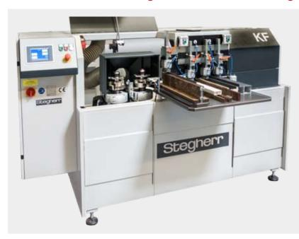
The Coping Center Stegherr KF is a machining center for cutting to length, milling, drilling and dowel driving in the window and door manufacturing industry.
